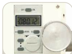
Quill Depth Digital Readout
