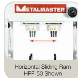
Dual Purpose Pressing Blocks HPF-50
