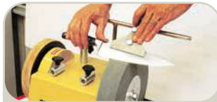
JIG 120 Designed for knives with blade length of 100 to 200mm
