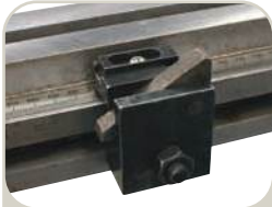
Flip Over Material Stop
