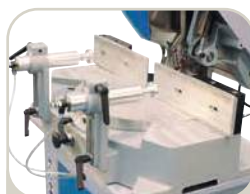
Dual Material Air Clamp System
