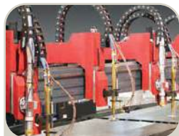
Multi-Head & Oxy Cutting Options
