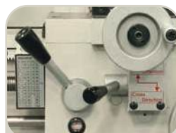
Feed Engage Lever AL-960B
