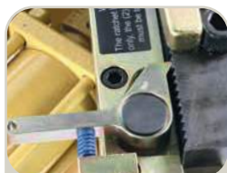
Ratcheting Counter Die Adjustment
