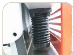
Hydraulic Material Hold Downs
