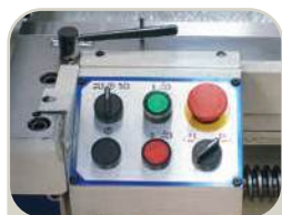
Saddle Switch Board
