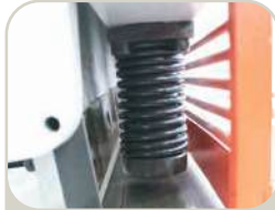
Hydraulic Material Hold Downs
