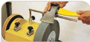
JIG 40 The perfect attachment for Axes with a blade up to 170mm
