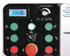
Control Panel With DRO HM-54GV
