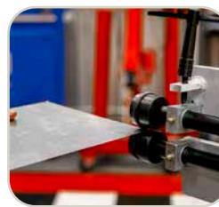
Top Roll Pressure Adjustment Handle
