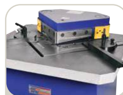
Adjustable Material Guides HN-220
